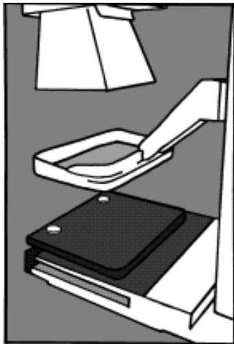
Fig. 2.3 Alignment of X-ray field/image receptor measurement
